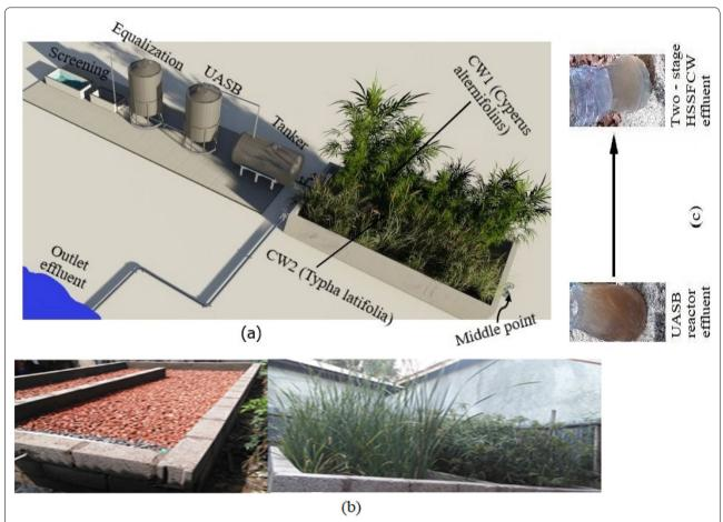
**Fig. 1** a Design of the two-stage HSSFCWs in treating UASB reactor effluent, **b** field view of the two-stage HSSFCW unit before planting and after plantation and **c** two-stage HSSFCW treated effluent quality
