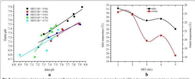
Fig. 2 a Correlation of inlet and outlet pH and **b** inlet and outlet temperature changes for each HRTs in the series-connected two-stage HSSFCW during the monitoring period
