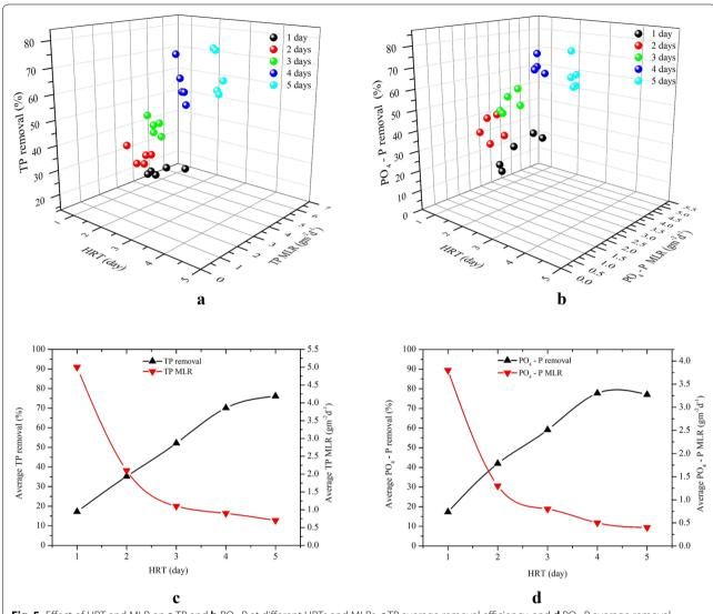
Fig. 5 Effect of HRT and MLR on **a** TP and **b** PO<sub>4</sub>-P at different HRTs and MLRs, **c** TP average removal efficiency, and **d** PO<sub>4</sub>-P average removal efficiency at different HRTs and MLRs in a two-stage HSSFCW
