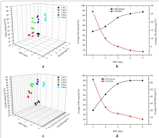
Fig.3 a Effect of HRT and MLR on TSS removal, **b** average TSS removals at different HRTs and MLRs, **c** effect of HRT and MLR on COD removal, and **d** average COD removals at different HRTs and MLRs in a series-connected two-stage HSSFCW. Dots indicate five rounds of sampling removals for each HRT
