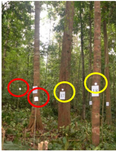
Fig. 3 Setting of circular (yellow color) and cylindrical (red color) reflectors in sample plots
