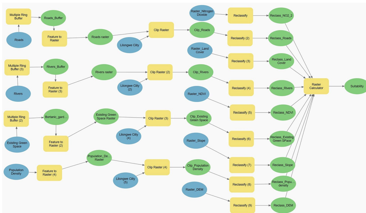
Fig. 3 Suitability for Green spaces implementation in Lilongwe City analysis workflow through ArcGIS Pro 3.3 Model Builder tool
