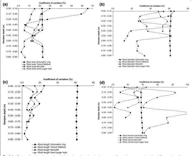
Fig. 6 Coefficients of variation by sampling depths in the evaluated methods **a** root area, **b** root diameter, **c** root length and **d** root volume (Source: The Authors (2021))
