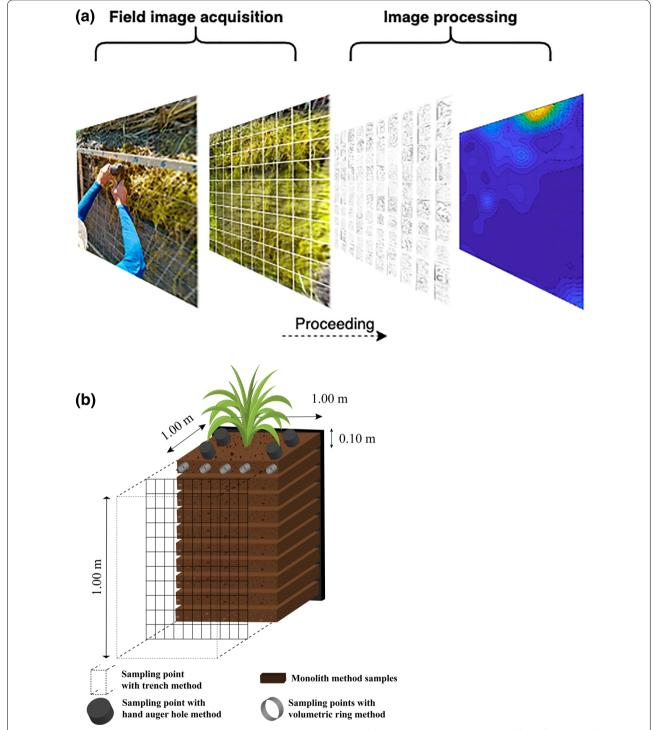
Fig. 2 a Roots and soil collection with the volumetric ring showing the insertion of the rings in the soil on the vertical face of the trench for sample collection and subsequent image processing; **b** Schematic diagram of the adopted methods for root collection (Source: The authors (2021))
