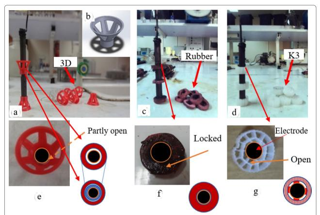
Fig. 5 Different microbial electrode jacket-dish (MEJ-dish) used during this study a 3D, b 3D design, c Rubber, d K3 MEJ-dish, and e-g junction between the electrode and MEJ-dish: partly opened (closed), open, and locked (closed). Locked (closed) indicates no space between the electrode and MEJ-dish, partly open shows the upper part is open, but the lower part is partially open or closed, and open means the connection part is exposed for microbial attachment
