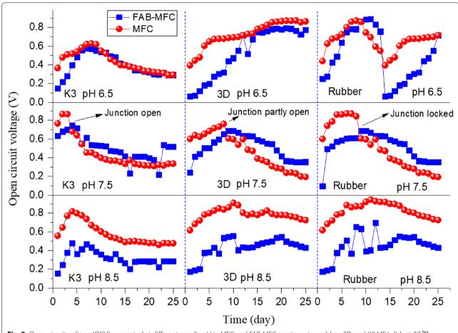
**Fig. 9** Open circuit voltage (OCV) generated at different anodic pH in MFC and FAB-MFC reactor using rubber, 3D, and K3 MEJ-dish at 27 °C. Junction refers to the space between the electrode and MEJ-dish (where MEJ-dish was connected to the electrode); K3 (open), 3D (partly opens), and rubber lock (close) the junction
