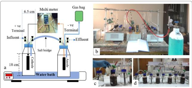
**Fig. 1** Double-chambered FAB-MFC optimization setup **a** schematic diagram, **b** photo, **c**, **d** during the construction of the reactors. The cylinder is the N<sub>2</sub> gas sparged into the anode reactors and hardcover laboratory notebook to record the results
