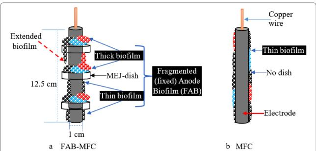
**Fig. 3** Conceptual scheme of electro-active biofilm (EABs) formation on **a** microbial electrode jacket-dish (MEJ-dish) in fragmented electro-active biofilm-microbial fuel cell (FAB-MFC) anode, and **b** without MEJ-dish in MFC anode
