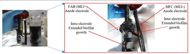
Fig. 7 Biofilm growth and development in bench-scale FAB-MFC setup. The biofilm extended in between the FAB (MEJ+) and MFC (MEJ-) anode electrode inserted in the same reactor
