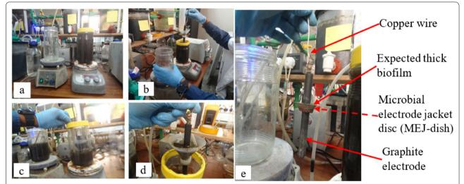
**Fig. 4** Fragmented electro-active biofilm (FAB) reactor conceptual scheme **a** raw domestic wastewater and inoculum fed into the reactor, **b** microbial electrode jacket dish (MEJ-dish) inserted to the graphite electrode, **c** pumping wastewater from the reactor, **d** removing the electrode, and **e** solid mass collected on the MEJ-dish
